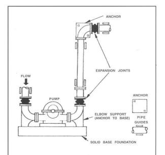
Typical Piping Layout Utilizing Expansion Joints (when equipment and piping are properly anchored)
